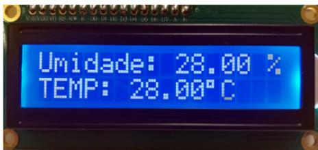
**Figura 4:** Display LCD 16x2 Backlight Azul
